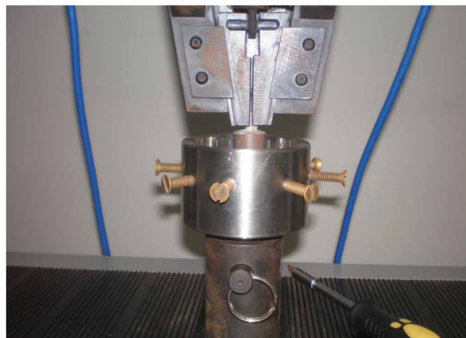
Figure 4. Pull-out strength test on a testing machine (KRATOS-IKCL-USB), at a speed of 0.5mm/min.
